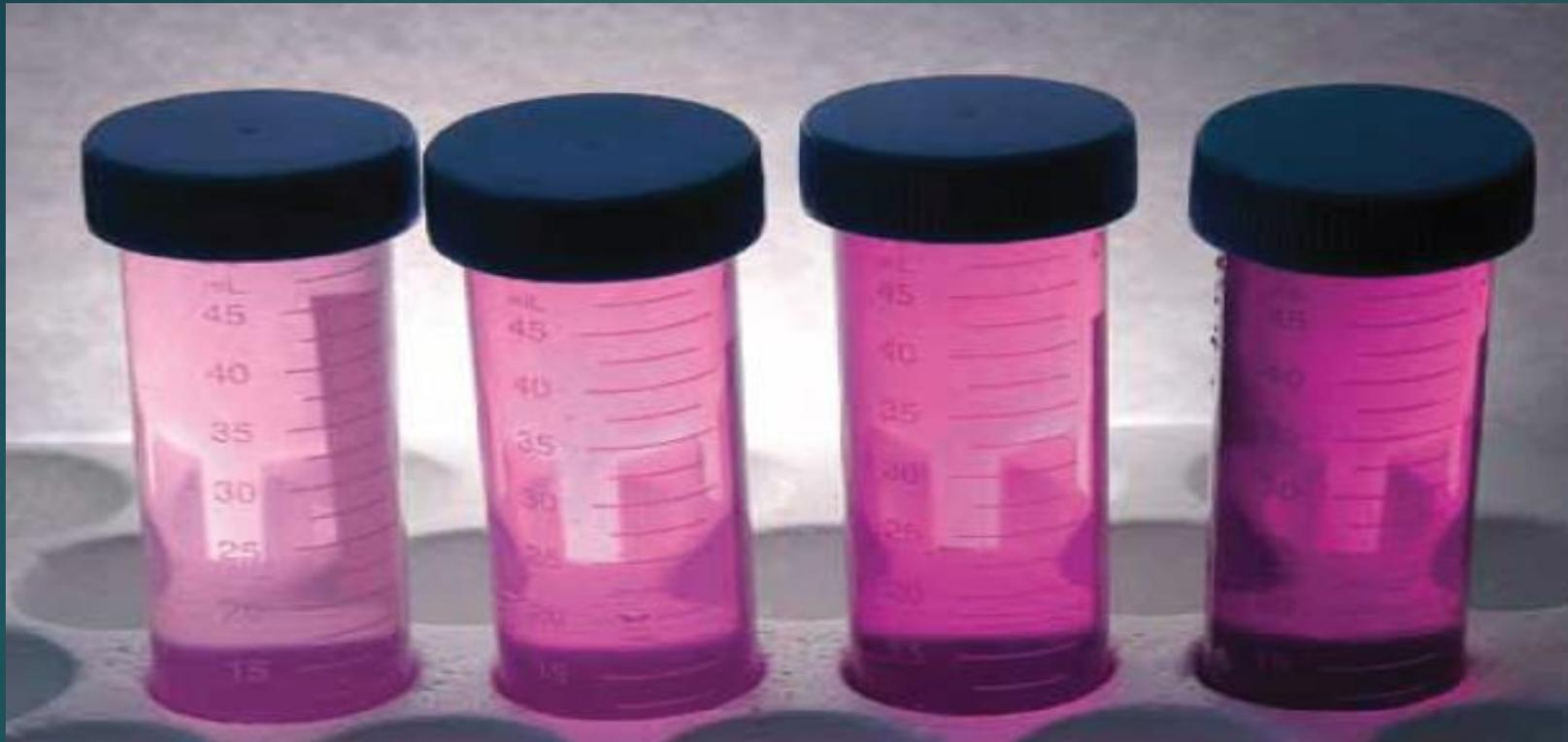
The test tubes shown here are laboratory standards for the POXC measurement, showing the range of values possible with permanganate oxidizable carbon (POXC). The lighter color is where more active carbon was oxidized, from a soil with more active carbon.
